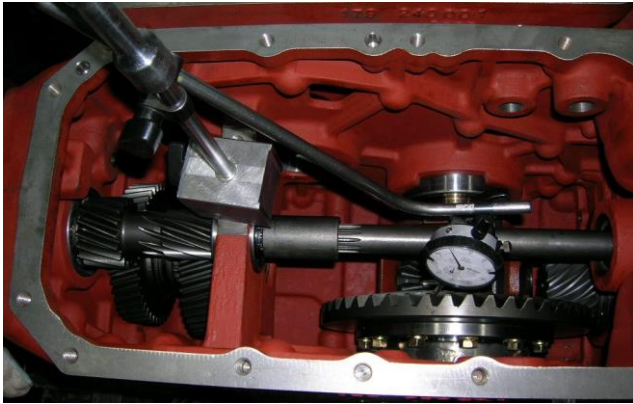
Adjust the shimming to backlash
